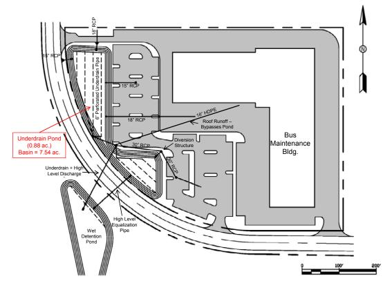
Figure 2-22. Drainage Features for the Orlando Underdrain Site.
