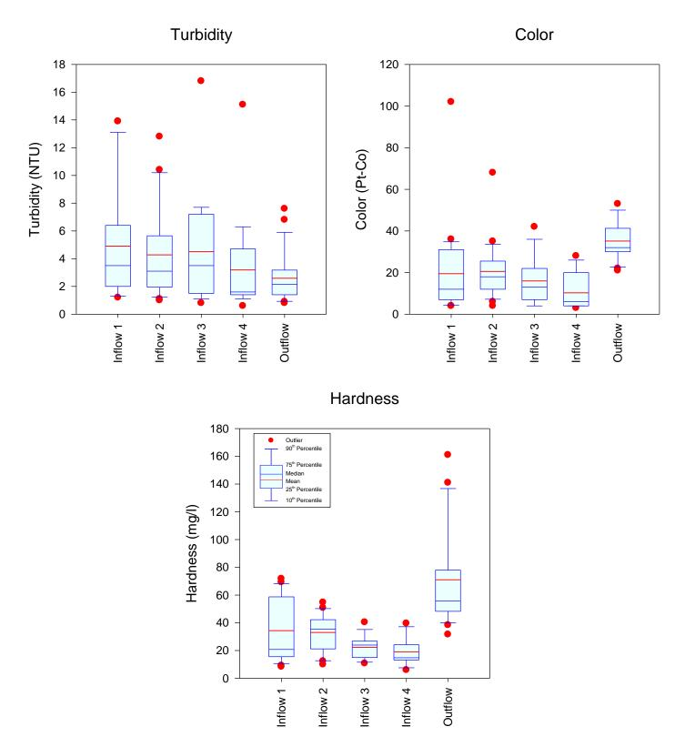
Figure 5-19. Statistical Comparison of Measured Values for Turbidity, Color, and Hardness at the Orlando Underdrain Site from December 2012-November 2013.
