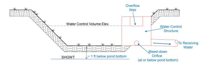
Figure 2-1. Schematic of a Typical Dry Detention Pond System.
