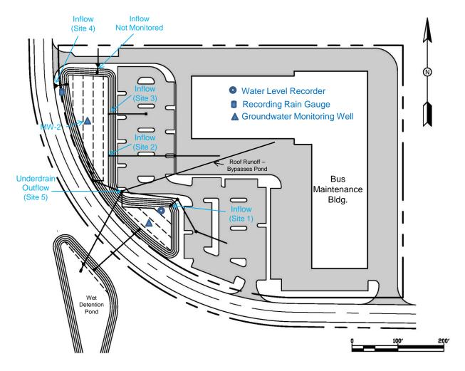
Figure 3-16. Overview of Field Monitoring Locations and Activities Conducted at the Orlando Underdrain Site.
