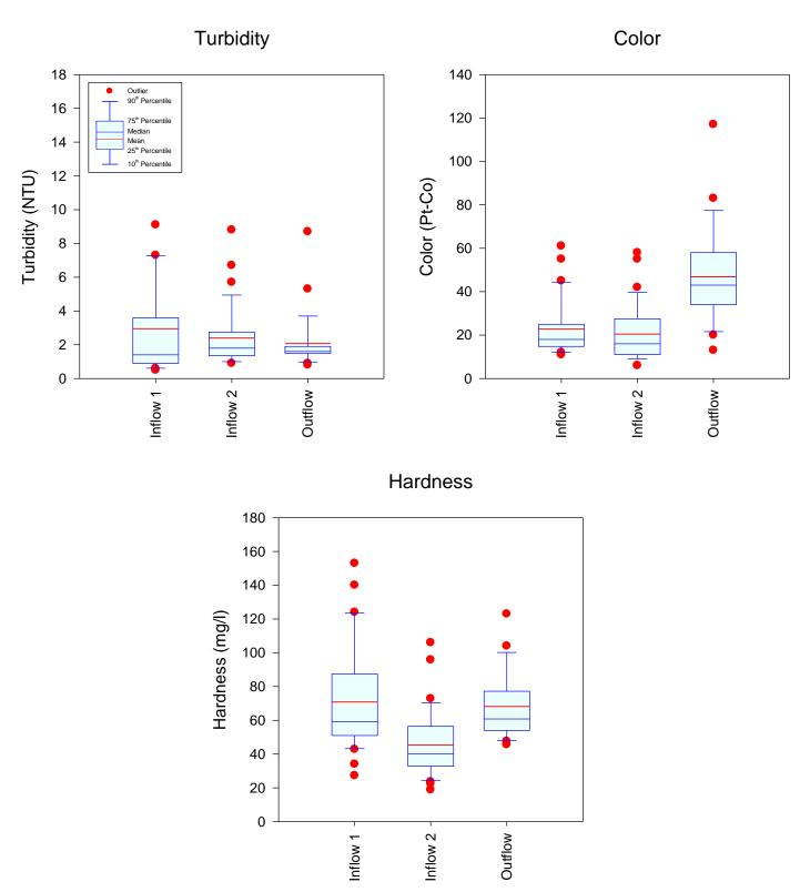
Figure 5-14. Statistical Comparison of Measured Values for Turbidity, Color, and Hardness at the Pembroke Pines Dry Detention Site from December 2012-November 2013.
