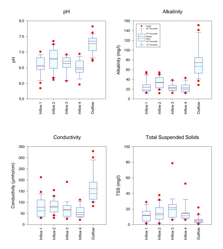
Figure 5-16. Statistical Comparison of Measured Values for pH, Alkalinity, Conductivity, and TSS at the Orlando Underdrain Site from December 2012-November 2013.
