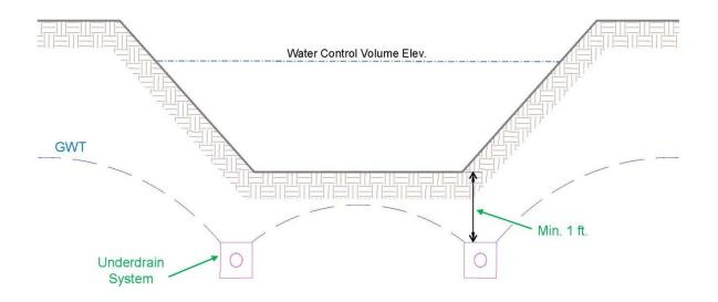
Figure 2-3. Schematic of a Typical Underdrain System.
