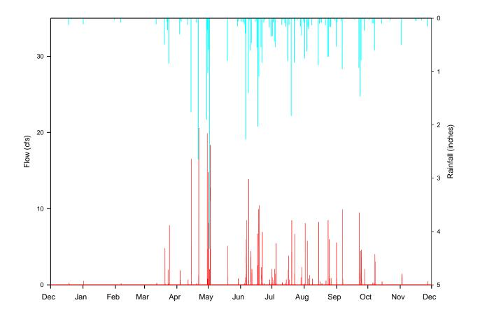
Figure 4-25. Measured Inflow Hydrographs at Orlando Underdrain Site 5 (Underdrain Outflow) from December 2012-November 2013.
