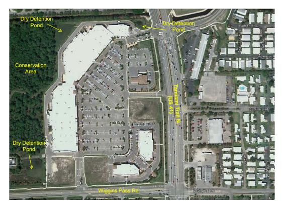
Figure 2-6. Overview of the Bonita Springs Dry Detention Site.
