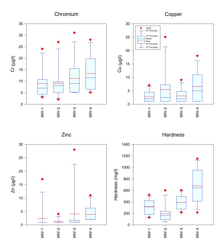
Figure 5-29. Statistical Comparison of Measured Concentrations of Chromium, Copper, Zinc, and Hardness in Groundwater at the Bonita Springs Site from December 2012-November 2013.
