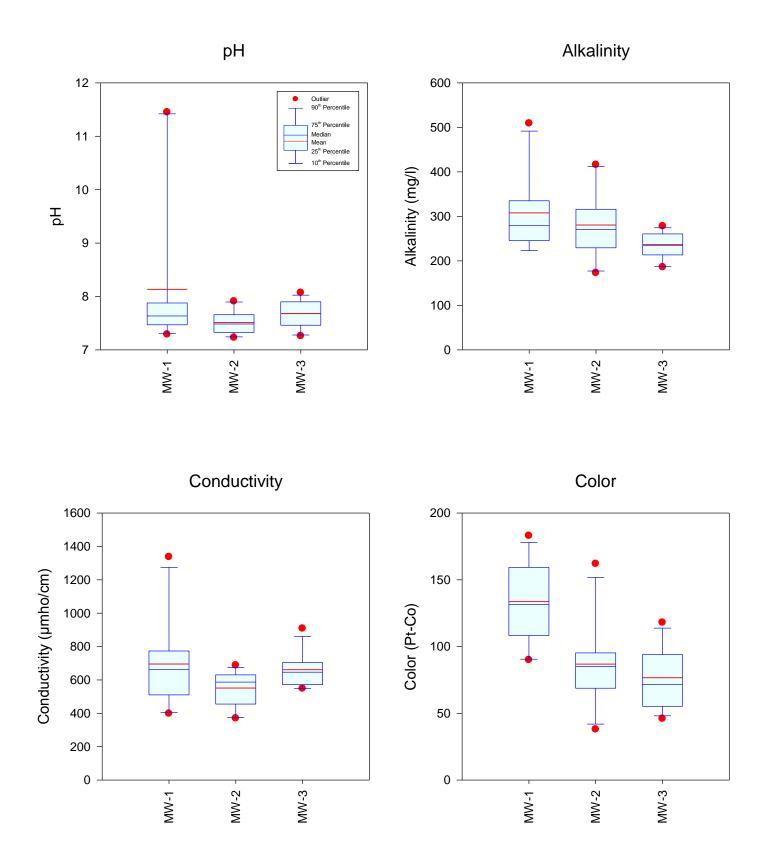
Figure 5-34. Statistical Comparison of Measured Values for pH, Alkalinity, Conductivity, and Color in Groundwater at the Pembroke Pines Site from December 2012-November 2013.
