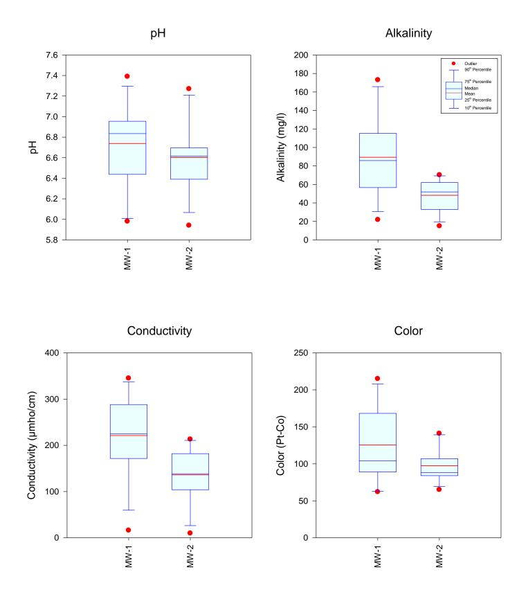
Figure 5-38. Statistical Comparison of Measured Values for pH, Alkalinity, Conductivity, and Color in Groundwater at the Orlando Underdrain Site from December 2012-November 2013.
