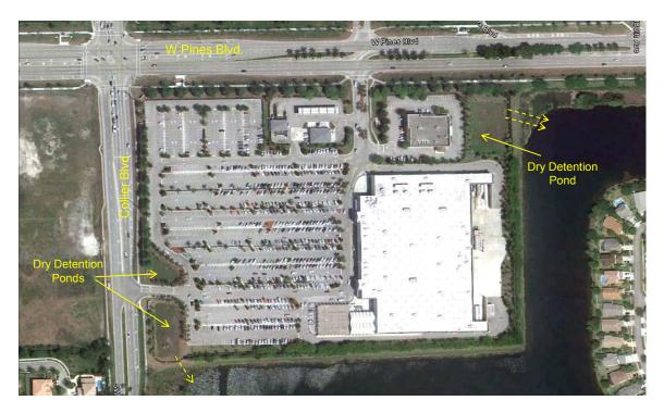
Figure 2-16. Overview of the Pembroke Pines Dry Detention Site.
