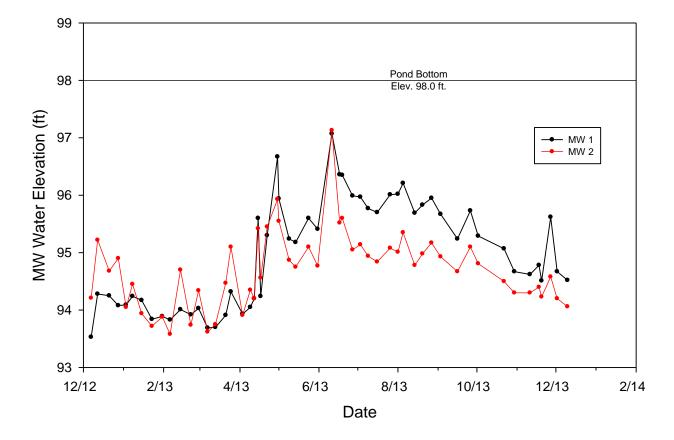
Figure 4-8. Measured Groundwater Elevations in the Underdrain Pond at the Orlando Site.
