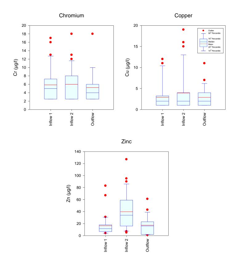
Figure 5-15. Statistical Comparison of Measured Concentrations of Chromium, Copper, and Zinc at the Pembroke Pines Dry Detention Site from December 2012-November 2013.
