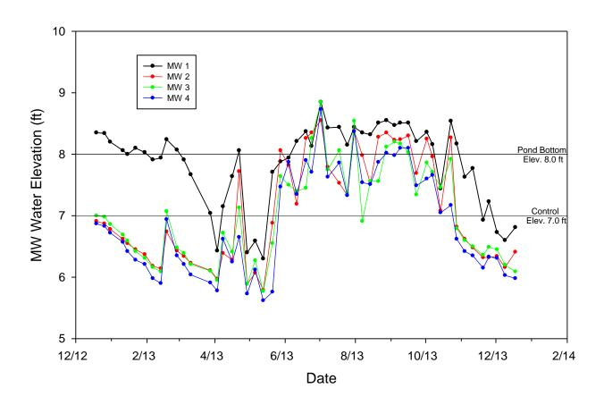
Figure 4-5. Measured Groundwater Elevations in the Dry Detention Ponds at the Bonita Springs Site.
