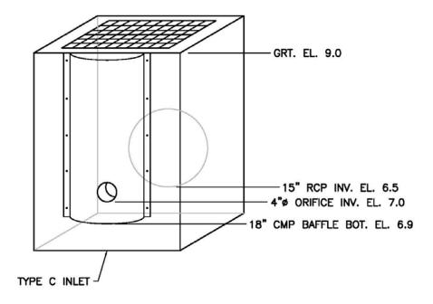
Figure 2-9. Schematic of the Outfall Structure for the Bonita Springs Dry Detention System.
