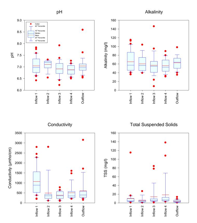
Figure 5-1. Statistical Comparison of Measured Values for pH, Alkalinity, Conductivity, and TSS at the Bonita Springs Dry Detention Site from December 2012-November 2013.
