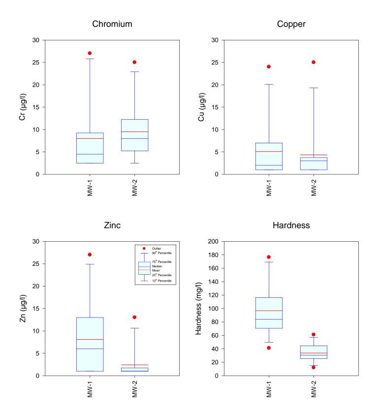
Figure 5-41. Statistical Comparison of Measured Concentrations of Chromium, Copper, Zinc, and Hardness in Groundwater at the Orlando Underdrain Site from December 2012-November 2013.
