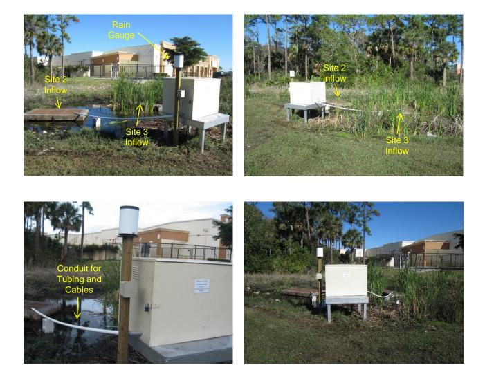
Figure 3-3. Photographs of Monitoring Equipment Installed at Bonita Springs Sites 2 and 3.
