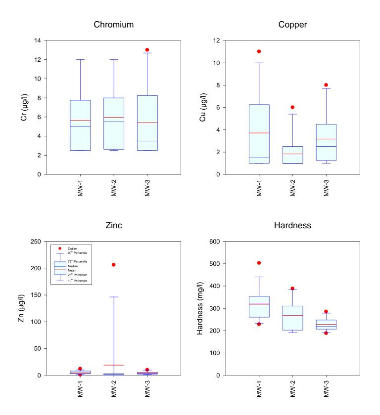
Figure 5-37. Statistical Comparison of Measured Concentrations of Chromium, Copper, Zinc, and Hardness in Groundwater at the Pembroke Pines Site from December 2012-November 2013.
