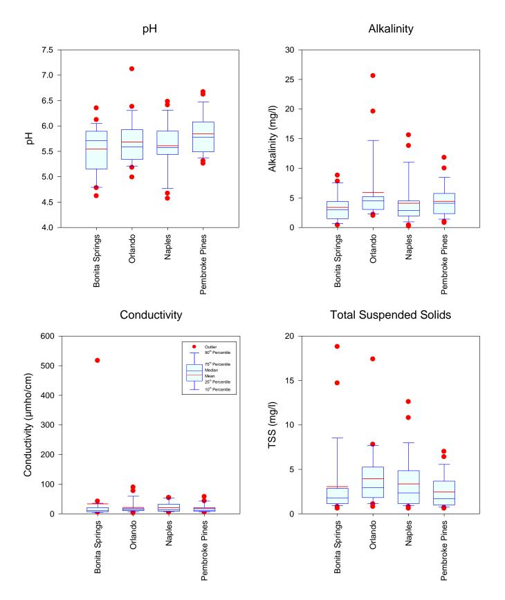
Figure 5-21. Statistical Comparison of Measured Values for pH, Alkalinity, Conductivity, and TSS at the Four Monitoring Sites from December 2012-November 2013.
