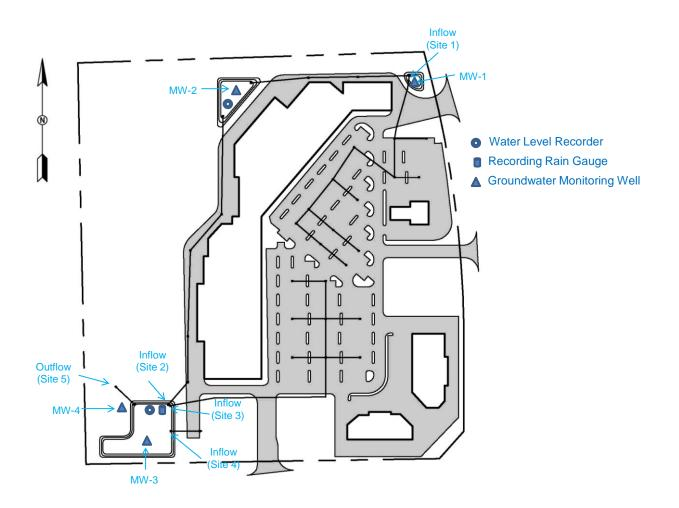
Figure 3-1. Overview of Field Monitoring Locations and Activities Conducted at the Bonita Springs Dry Detention Pond Site.
