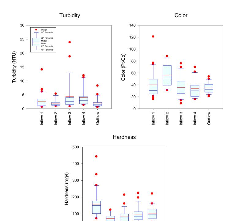
Figure 5-4. Statistical Comparison of Measured Values for Turbidity, Color, and Hardness at the Bonita Springs Dry Detention Site from December 2012-November 2013.
