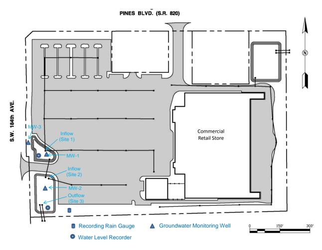
Figure 3-12. Schematic of Monitoring Locations and Hydrologic Instrumentation Used at the Pembroke Pines Dry Detention Pond Site.
