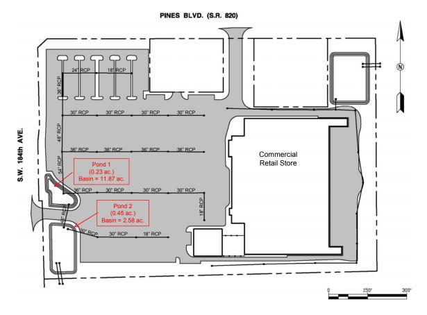
Figure 2-17. Drainage Features for the Pembroke Pines Dry Detention Site.
