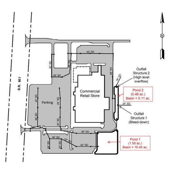
Figure 2-12. Drainage Features for the Naples Dry Detention Site.
