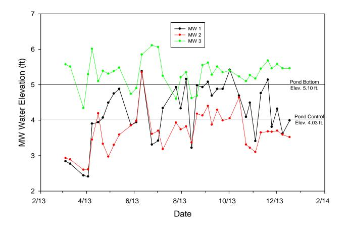
Figure 4-7. Measured Groundwater Elevations in the Dry Detention Ponds at the Pembroke Pines Site.
