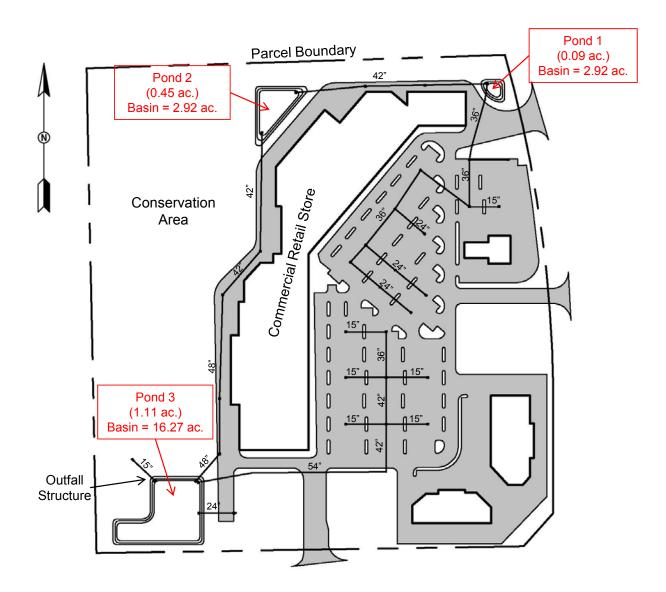
Figure 2-7. Drainage Features for the Bonita Springs Dry Detention Site.
