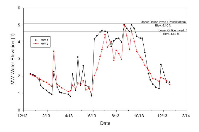
Figure 4-6. Measured Groundwater Elevations in the Dry Detention Ponds at the Naples Site.
