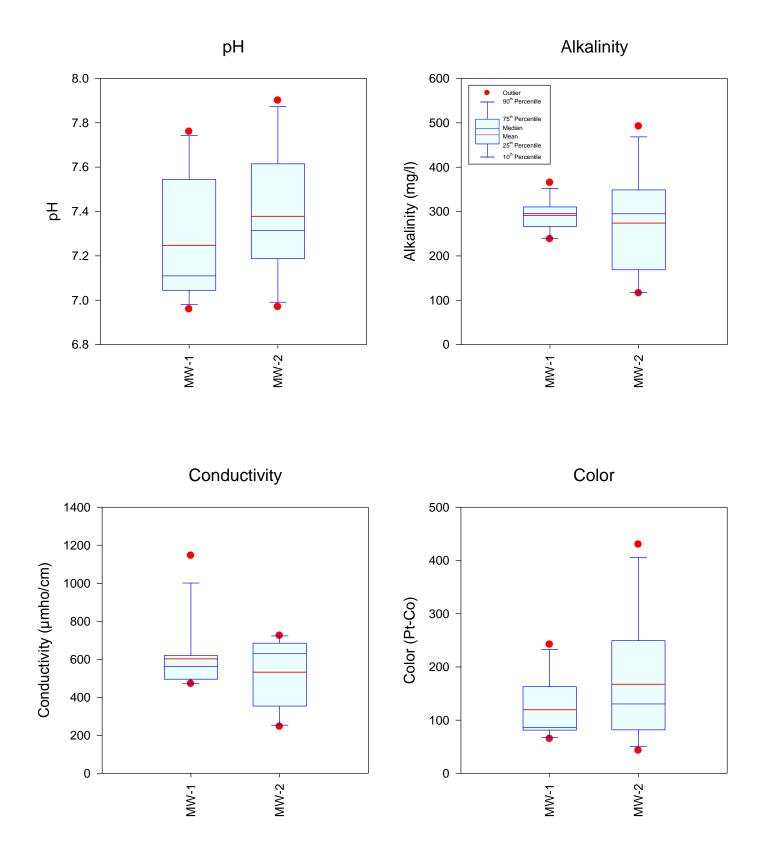
Figure 5-30. Statistical Comparison of Measured Values for pH, Alkalinity, Conductivity, and Color in Groundwater at the Naples Site from December 2012-November 2013.
