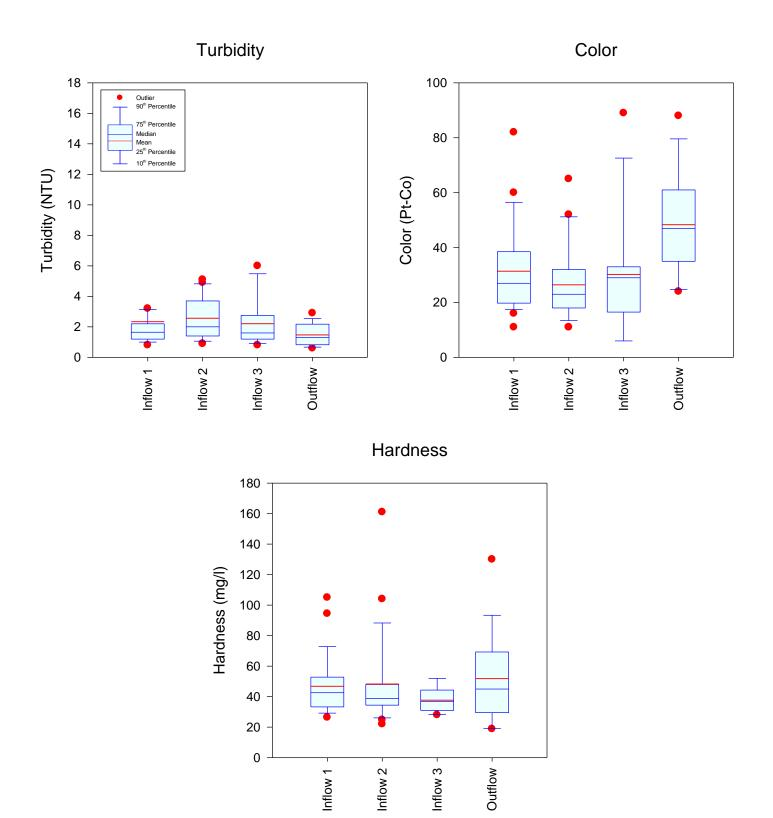
Figure 5-9. Statistical Comparison of Measured Values for Turbidity, Color, and Hardness at the Naples Dry Detention Site from December 2012-November 2013.
