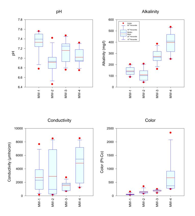
Figure 5-26. Statistical Comparison of Measured Values for pH, Alkalinity, Conductivity, and Color in Groundwater at the Bonita Springs Site from December 2012-November 2013.
