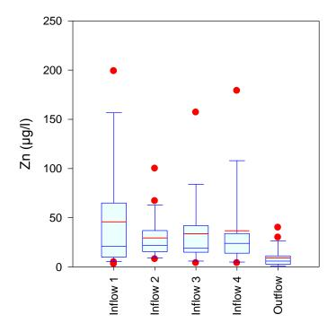
Figure 5-20. Statistical Comparison of Measured Concentrations of Chromium, Copper, and Zinc at the Orlando Underdrain Site from December 2012-November 2013.
