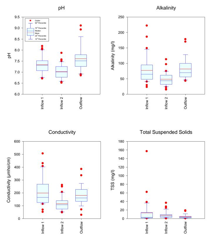
Figure 5-11. Statistical Comparison of Measured Values for pH, Alkalinity, Conductivity, and TSS at the Pembroke Pines Dry Detention Site from December 2012-November 2013.
