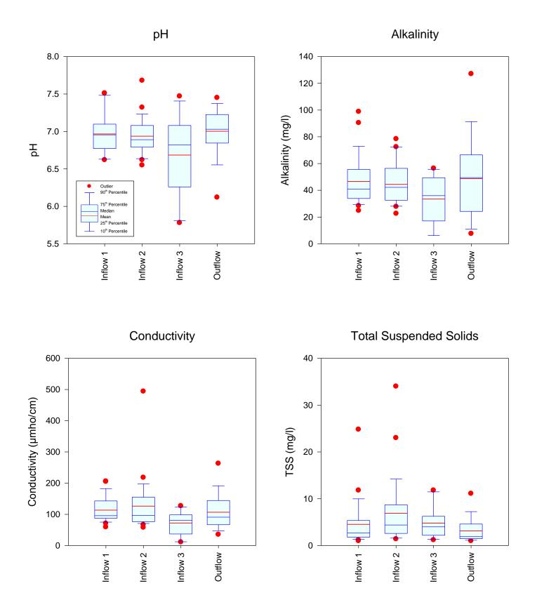
Figure 5-6. Statistical Comparison of Measured Values for pH, Alkalinity, Conductivity, and TSS at the Naples Dry Detention Site from December 2012-November 2013.
