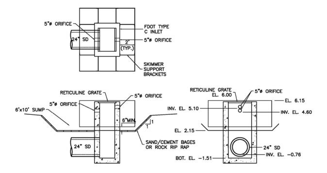
Figure 2-14. Overview of Outfall Structure 1 at the Naples Dry Detention Site.
