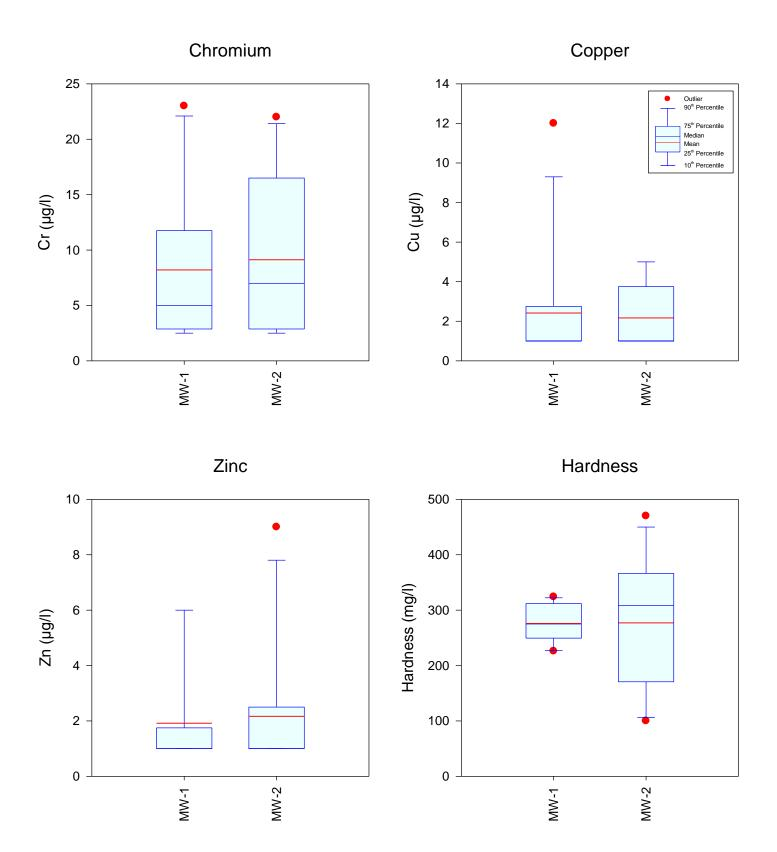
Figure 5-33. Statistical Comparison of Measured Concentrations of Chromium, Copper, Zinc, and Hardness in Groundwater at the Naples Site from December 2012-November 2013.
