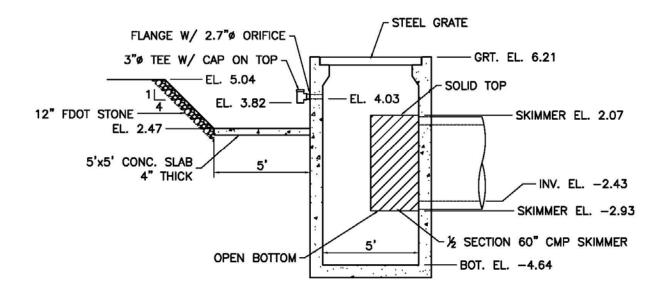
Figure 2-19. Overview of the Outfall Structure for Pond 2 at the Pembroke Pines Site.
